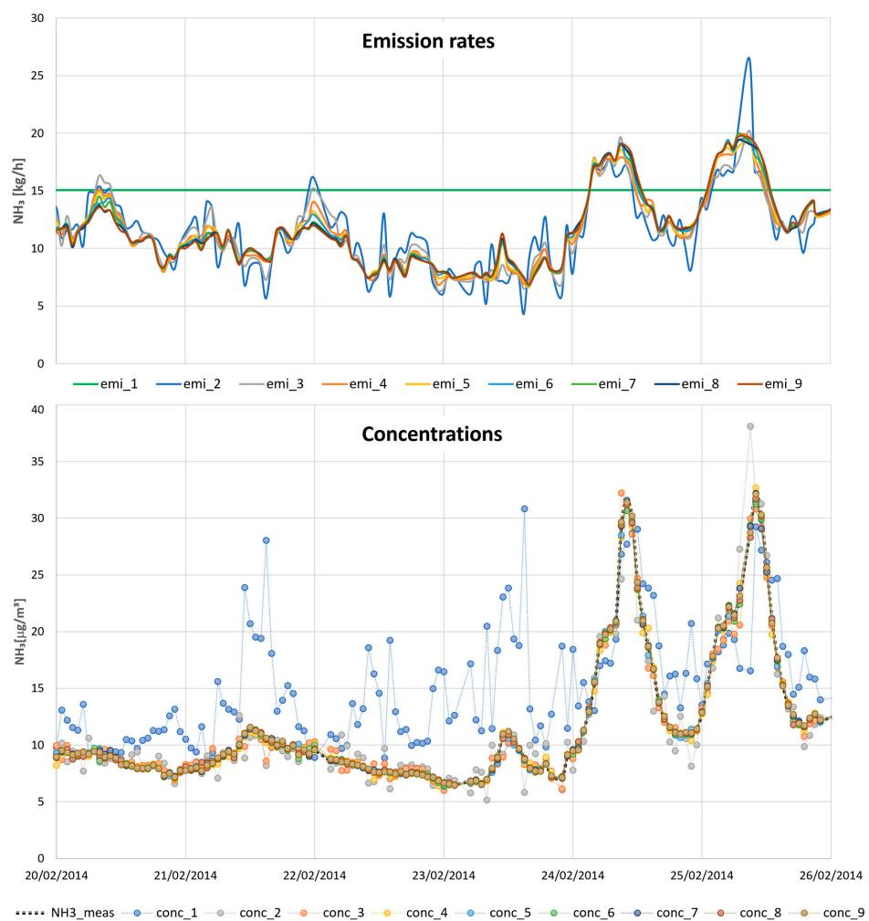
**Figure 2.** Focus on a short period for station 10\_RB. Emission rates: illustrate the variation in the estimated emission flux for each model iteration. Concentrations: comparison between the predicted and measured concentrations of  $\text{NH}_3$  for each model iteration.
