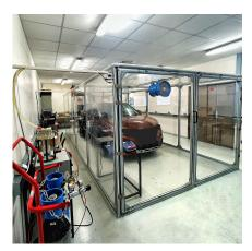
Figure 1. Closed chamber (the bubble) for outdoor air control and vehicle in-cabin preconditioning.
