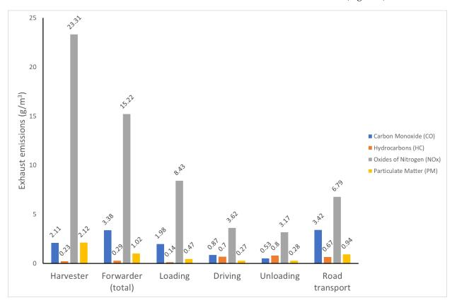
**Figure 2.** Exhaust emissions for individual timber extraction stages for 1 m<sup>3</sup> of timber adapted from [59].
