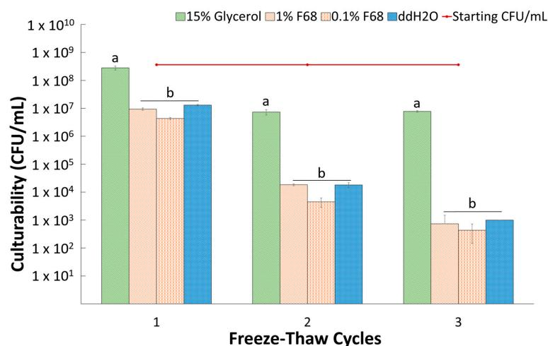
**Figure 6.** Effect of freeze/thaw cycles in an automated freezer on culturability of *PcO6*. The data show the mean of culturable cells/mL obtained on LB agar after 1, 2, or 3 freeze/thaw cycles. Error bars are the standard deviations of three replicates. Letters denote significant ( $p < 0.01$ ) differences among treatments for a given free/thaw cycle using one-way ANOVA followed by Tukey's HSD.
