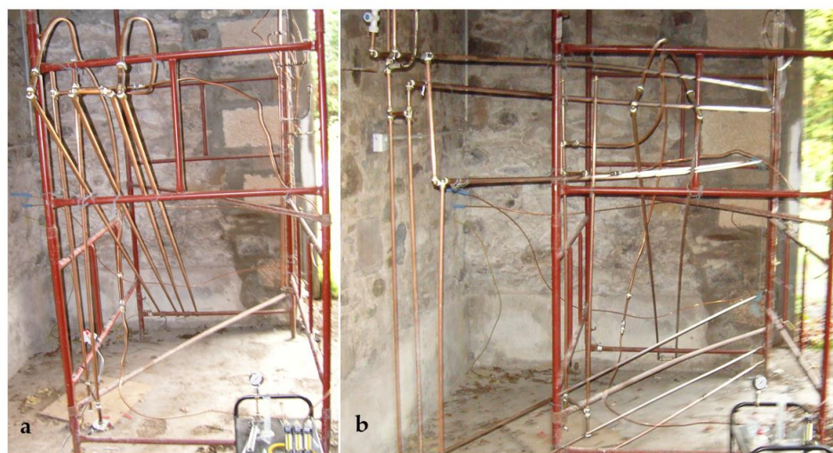
Figure 9. Reactor configuration: (a) FBR containing a 12 m particulate column; (b) configuration used in this study of a FBR constructed from two 3 m-long pipe segments and the BCDR. Note the pipe sections which have a white colour. These are sections which are associated with significant hydrogen discharge through the pipe wall.
