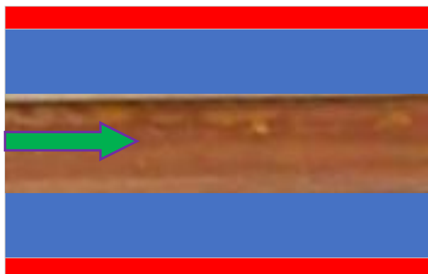
Figure 4. Design concept. Copper central tubing: inner shell and inner annulus. Blue = outer annulus of the outer shell. It receives hydrogen through the wall of the inner shell from the inner annulus. Red = bunding shell of the reactor. Arrow indicates direction of gas flow within the inner annulus.
