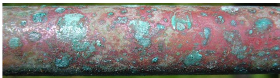
Figure 3. 15 mm O.D. copper pipe showing the effects of hydrogen leakage when the pipe (rated to 2 MPa water pressure) is pressured with a gas containing hydrogen at 0.1 to 0.3 MPa. Blue-green patches are formed by Cu(OH) x as the hydrogen reacts with both oxygen in the air and the Cu 0 at leakage points.
