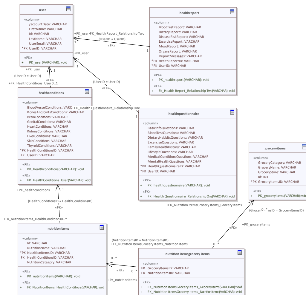
Figure 9. Physical Data Model for a health technology system.
