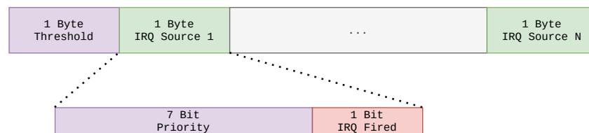
**Figure 3.** Mapping of fuzzer generated byte stream onto the PLIC functionality.
