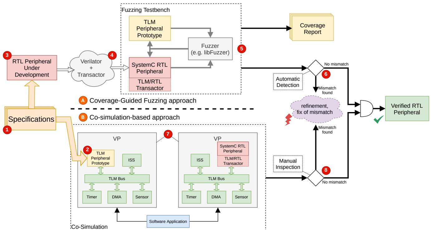
Figure 2. Overview of the cross-level methodology employed for the RTL/TLM development.
