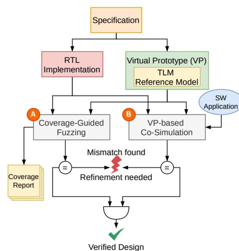
**Figure 1.** High level overview of our proposed Cross-Level Methodology.
