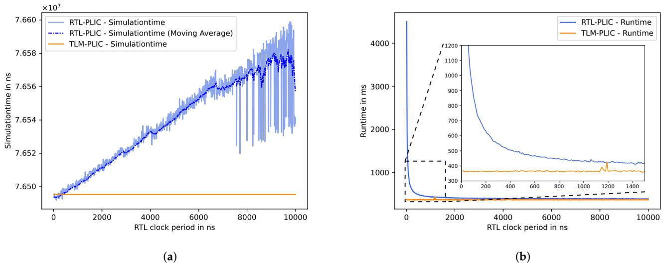
**Figure 4.** Performance comparison of VP executions with TLM and RTL PLIC respectively. (a) Internal simulation time against clock period of RTL PLIC; (b) Host execution time in relation to clock period of RTL PLIC.
