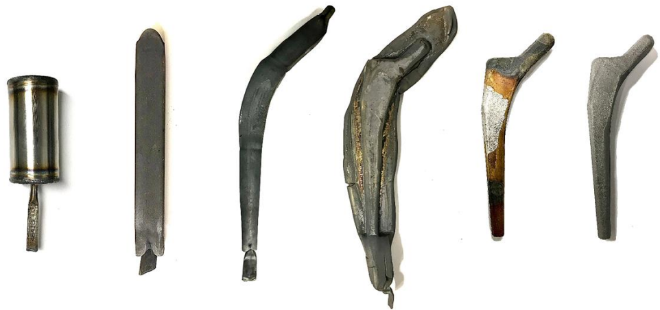
Figure 3. From left to right, photographs presenting the initial canister, the forged billet, the preform, the final precision forging, the cut-out sample and the sandblasted final component.
