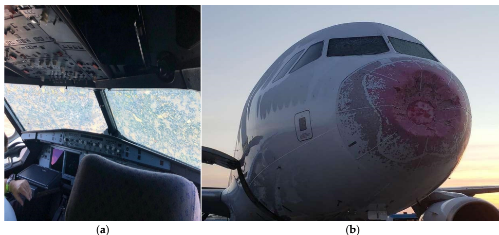
Figure 2. Aircraft structural damages after its encounter with MCC. (a) View from the cockpit. (b) External view [19].
