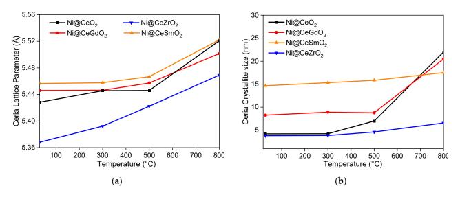
Figure 3. Variation of (a) ceria lattice parameter and (b) ceria crystallite size during reduction process.
