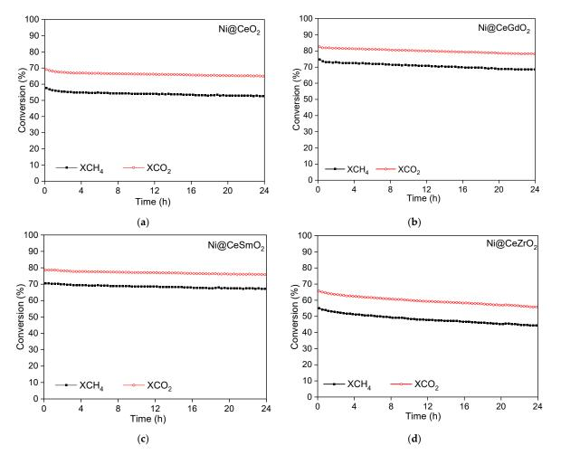
**Figure 8.** Conversion of CH<sub>4</sub> and CO<sub>2</sub> in the DRM at 800 °C as a function of TOS (CH<sub>4</sub>/CO<sub>2</sub> molar ratio of 1.0; W/F = 0.2 g<sub>cat</sub>·L<sup>-1</sup>h<sup>-1</sup>) for (a) Ni@CeO<sub>2</sub>, (b) Ni@CeGdO<sub>2</sub>, (c) Ni@CeSmO<sub>2</sub> and (d) Ni@CeZrO<sub>2</sub>.
