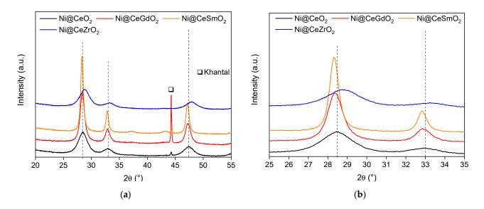
**Figure 1.** XRD patterns of fresh samples at room temperature: (a)  $2\theta = 20-55^{\circ}$ ; (b)  $2\theta = 25-35^{\circ}$ .
