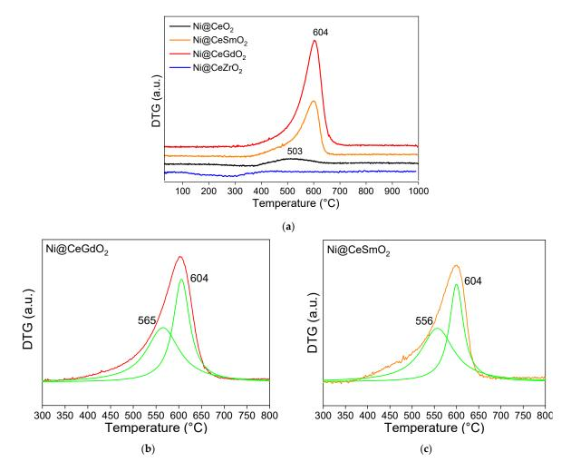
**Figure 10.** DTG profiles of (**a**) all used catalysts after DRM at 800  $^{\circ}$ C for 24 h of TOS with decomposition of the profiles for (**b**) Ni@CeGdO<sub>2</sub> and (**c**) Ni@CeSmO<sub>2</sub>.
