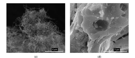
**Figure 11.** SEM images of spent catalysts after DRM at 800 °C for 24 h of TOS: (**a**) Ni@CeO<sub>2</sub>, (**b**) Ni@CeGdO<sub>2</sub>, (**c**) Ni@CeSmO<sub>2</sub> and (**d**) Ni@CeZrO<sub>2</sub>.
