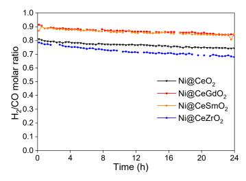
**Figure 9.**  $H_2/CO$  molar ratio obtained in the the DRM at 800 °C as a function of TOS (CH<sub>4</sub>/CO<sub>2</sub> molar ratio of 1.0; W/F = 0.2 g<sub>cat</sub>·L<sup>-1</sup>h<sup>-1</sup>).
