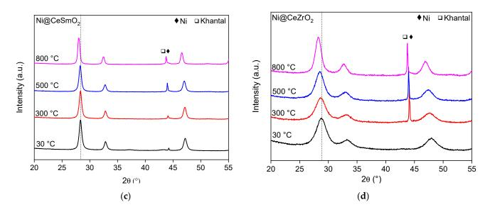
**Figure 2.** In-situ diffractograms obtained during reduction of (**a**) Ni@CeO<sub>2</sub>, (**b**) Ni@CeGdO<sub>2</sub>, (**c**) Ni@CeSmO<sub>2</sub> and (**d**) Ni@CeZrO<sub>2</sub>.
