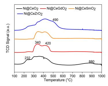
Figure 5. TPR profiles for the catalysts.
