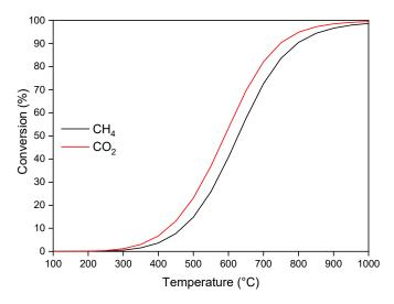
Figure 7. Reactant conversion and  $H_2/CO$  molar ratio at the thermodynamic equilibrium of the DRM reaction assuming no carbon formation.
