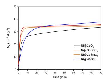
**Figure 6.** Evolution of the number of exchanged oxygen atoms during IOIE at 400 °C for Ni@CeO<sub>2</sub>, Ni@CeGdO<sub>2</sub>, Ni@CeSmO<sub>2</sub> and Ni@CeZrO<sub>2</sub>.
