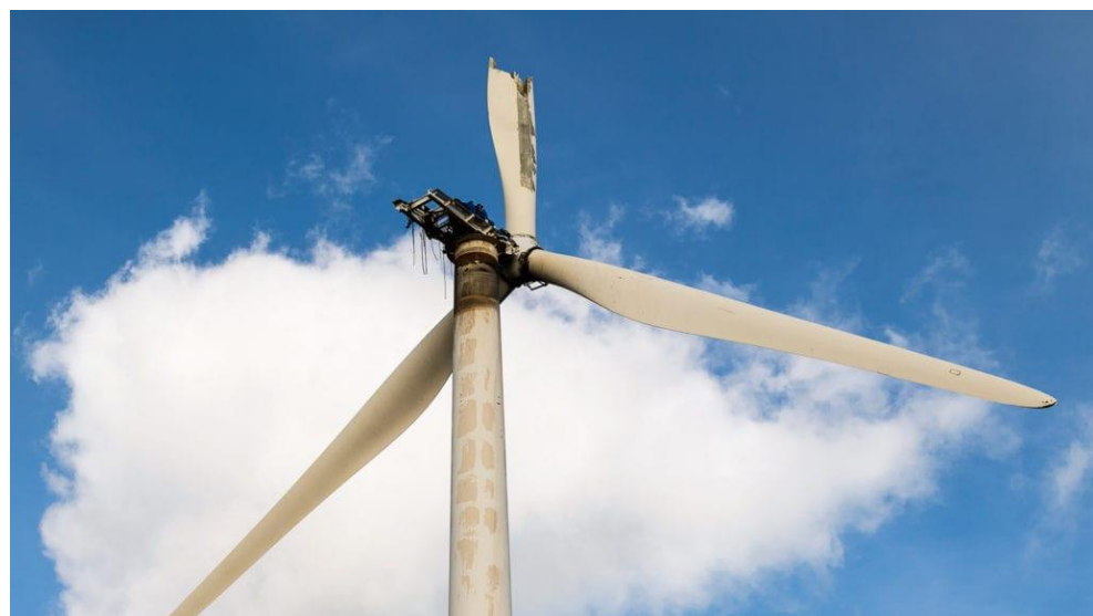
Figure 2. Severe wind turbine damage due to lightning [16].
