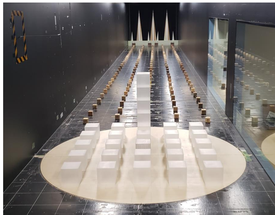
Figure 3. Photo of the experimental models installed in the wind tunnel of Case 1.
