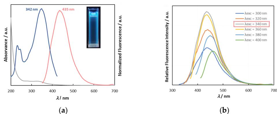
**Figure 1.** (a) UV-Vis spectra (gray), excitation (blue, monitored at 435 nm), and emission (orange;  $\lambda_{\text{exc}} = 340\text{ nm}$ ) of  $\mu$ Algae-CNDs in aqueous dispersion ( $0.1\text{ mg mL}^{-1}$ ) (inset: UV light at 366 nm); (b) Fluorescence emission spectra of  $\mu$ Algae-CNDs in aqueous dispersion ( $0.1\text{ mg mL}^{-1}$ ) with different excitation wavelengths. The red dashed line emphasize the excitation wavelength that has the highest intensity.
