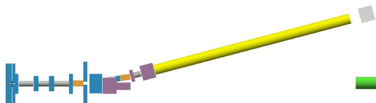
**Figure 1.** Latest beamline design. Focusing quadrupoles and bending dipoles are shown in gray and orange, respectively. Collimators are made of Iron (blue) or Inermet180 (violet). The decay tunnel (yellow), the hadron dump (light grey) and the proton dump (green) are also shown.
