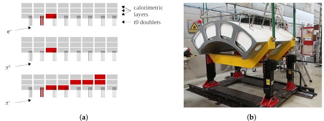
**Figure 3.** (a) Event topology for the ENUBET calorimeter. EM shower from a positron, top; EM shower from a  $\pi^0$ , middle; hadronic shower from a  $\pi^+$ , bottom. The modules involved in a typical  $e^+$ ,  $\pi^0$  or  $\pi^+$  event are marked in red. In the  $\pi^0$  case, photons coming from its decay do not leave any signal in the t0 doublet. (b) The demonstrator.
