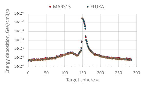
**Figure 3.** Energy deposition in W spheres as simulated with MARS15 and FLUKA. Target sphere # refers to the target sphere sequential number.
