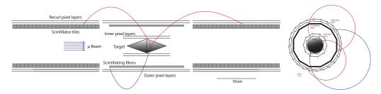
**Figure 2.** Schematic of the Mu3e phase I detector shown (**left**) along the beam axis and (**right**) transverse to the beam axis. A potential  $\mu^+ \to e^+e^-e^+$  signal decay is shown with  $e^+$  trajectories in red and the  $e^-$  trajectory in blue.
