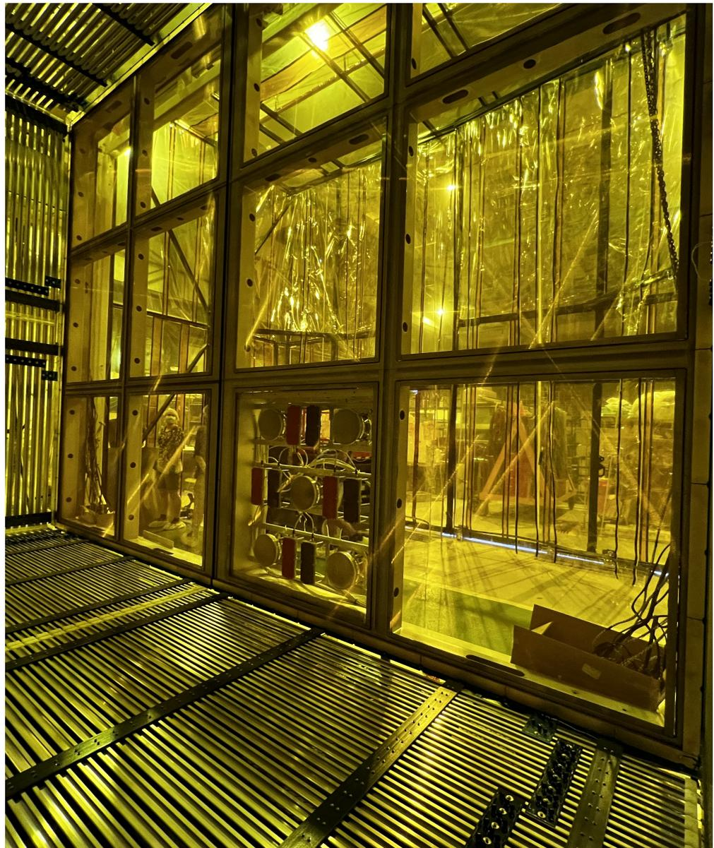
**Figure 4.** Picture of the right-hand-side TPC during the PDS installation, showing one of the PDS modules installed behind the APA.
