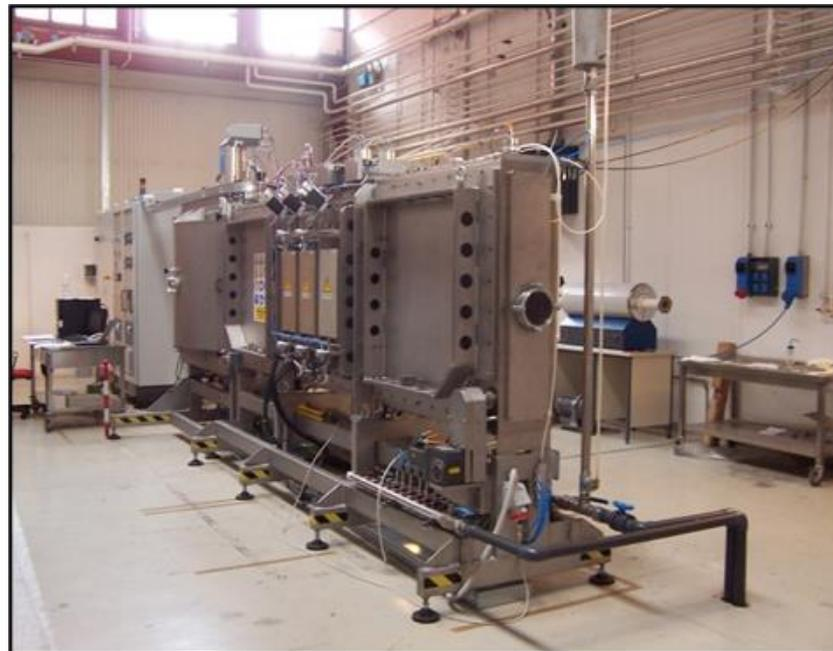
**Figure 1.** A general view of ENEA-2 sputtering plant.
