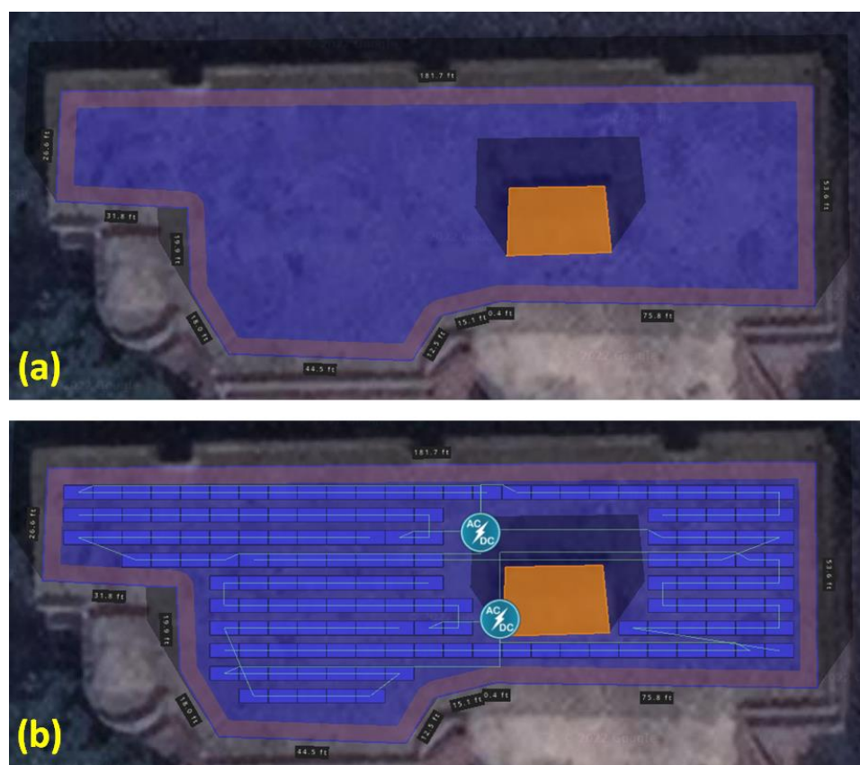
Figure 7. Images of rooftop space of the north block of the Udayan school, Dhaka (a) and the PV sizing obtained using the HelioScope simulation tools (b).
