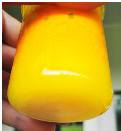
Figure A1. A hydrogel-based suspoemulsion with bead-milled curcumin four weeks after its production. The suspoemulsions with sonofragmented or bulk curcumin do not differ macroscopically from the picture shown.
