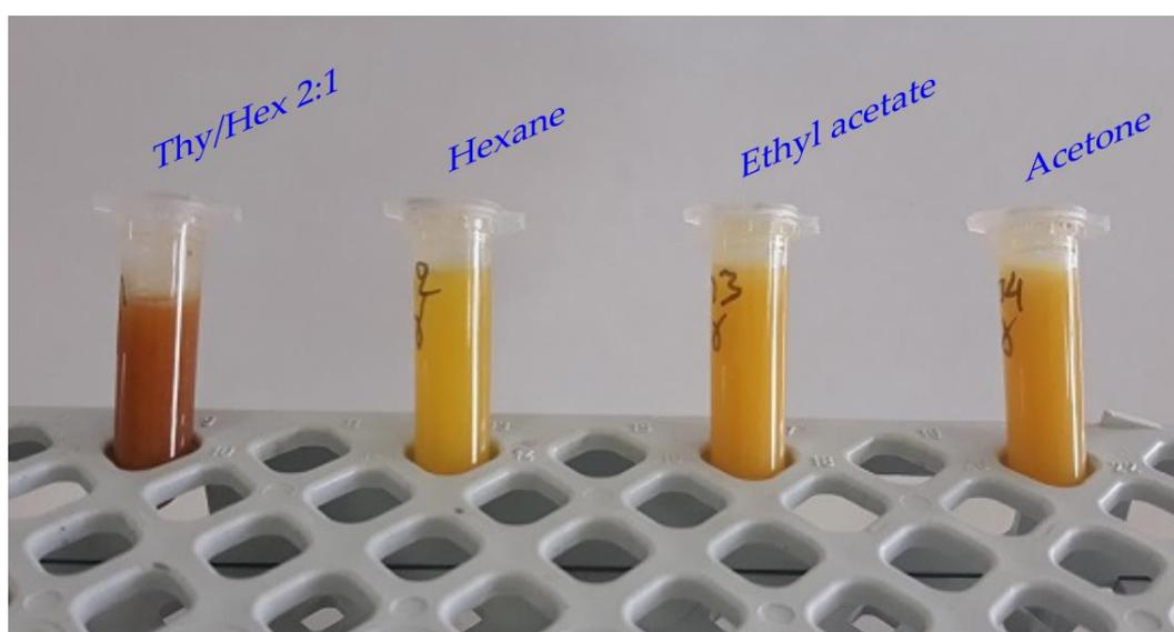
**Figure 3.** Extracts obtained with Thy/Hex 2:1, hexane, ethyl acetate, and acetone (from left to right) at optimum conditions.
