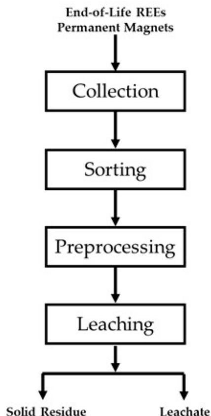
**Figure 2.** Flowsheet of the permanent magnet hydrometallurgical process.
