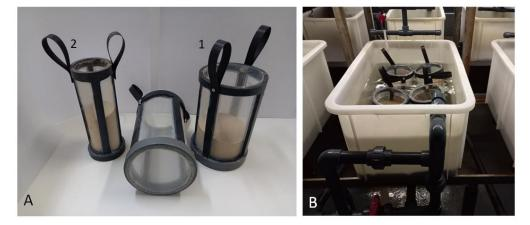
**Figure 1.** (**A**) Experimental units (EUs) for rearing polychaetes in trials 1 and 2. (**B**) Polycarbonate trays in which experimental units were placed.
