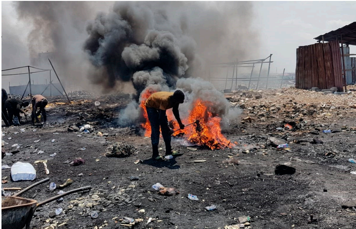
Figure 1. Recovery of desirable e-waste materials after burning plastic coatings.
