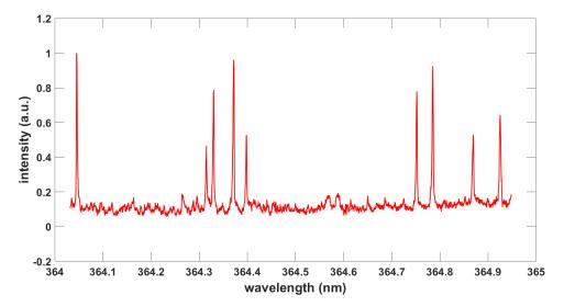
Figure 5. Recorded CH B–X spectrum using CRDS.
