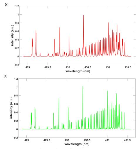
**Figure 3.** Comparison of measured (a) and fitted (b) CH A–X spectra,  $\delta \lambda = 0.005$  nm, T = 1.47 kK.
