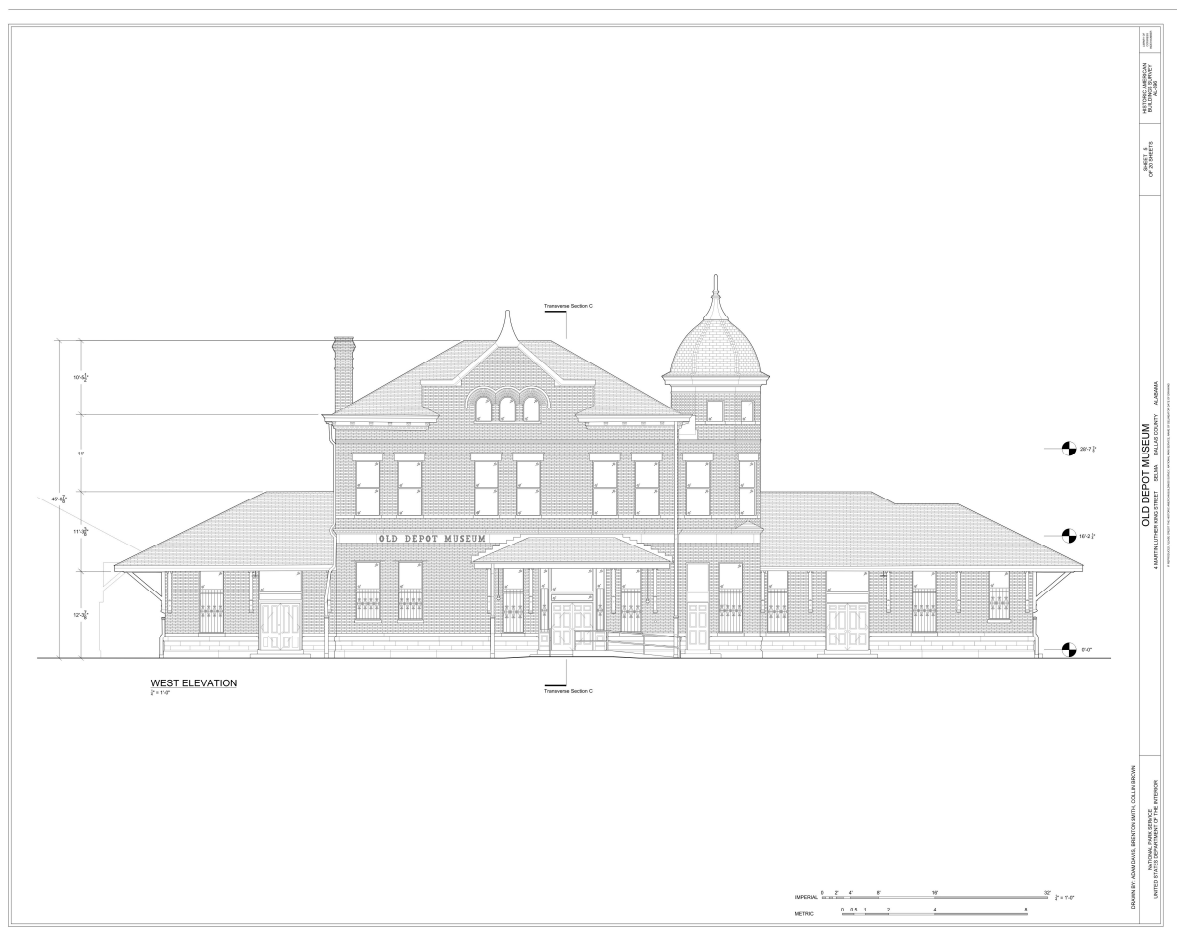
Figure 6. A front elevation of the Old Depot Museum was created using the TLS PC.
