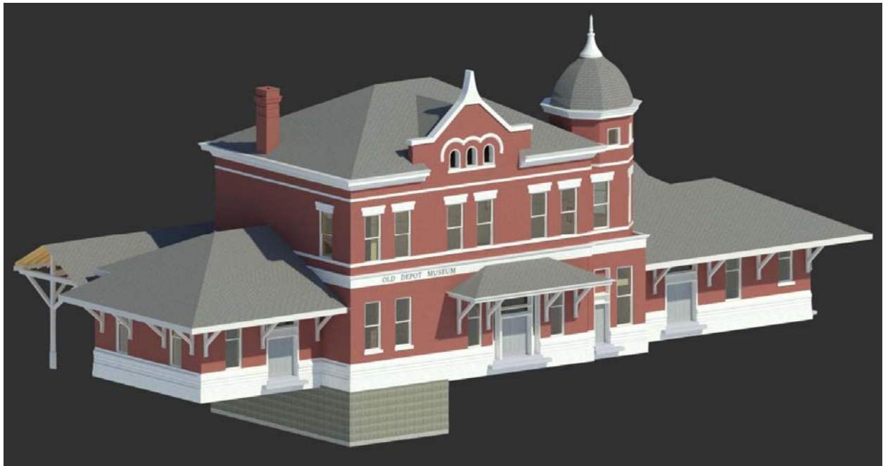
Figure 5. An HBIM model of the Old Depot Museum was developed using the TLS PC.
