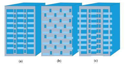
**Figure 4.** Various types of facade arrangement in high-rise buildings: (**a**) aligned balconies, (**b**) staggered balconies, (**c**) side balconies.
