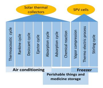
Figure 3. Different types of solar cooling systems.
