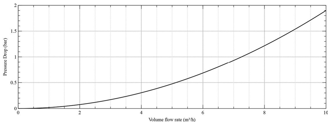
**Figure 5.** Pressure drop as a function of the feed volume flow rate (underflow rate = 0). Through multiplication of the pressure drop and the volume underflow rate of each set point, the energy consumption of the hydrocyclone can be estimated. For a typical setpoint (5 m<sup>3</sup>/h), the power consumption of the hydrocyclone is 66 W (simplified consideration neglecting individual coefficients of performance).
