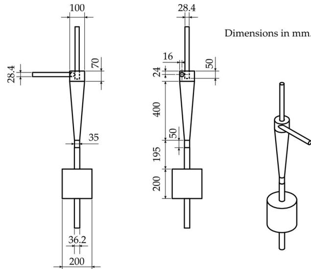
**Figure 3.** Hydrocyclone dimensions on the basis of a previous empirical study [26] with variation of the inlet diameter, vortex-finder diameter, vortex-finder length, cone angle and underflow configurations.
