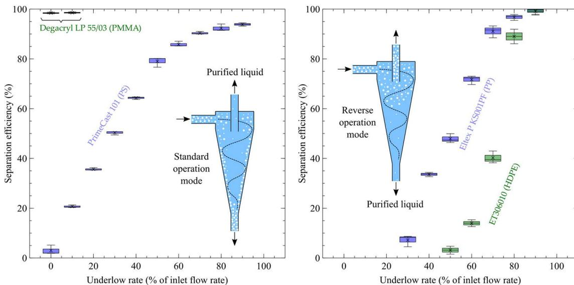
**Figure 4.** Standard (left) and reverse mode (right) operations of the hydrocyclone ( $5 \text{ m}^3/\text{h}$  inlet flow rate) with selected polymers and variation of the underflow rate.
