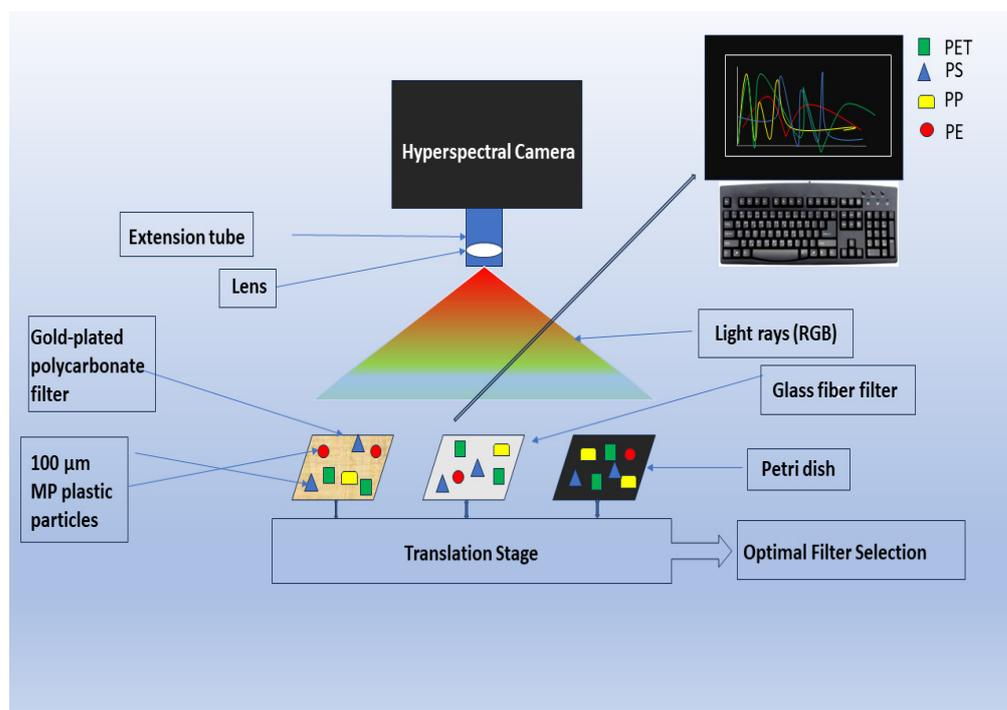
**Figure 3.** Framework of hyperspectral imaging for MP analysis.
