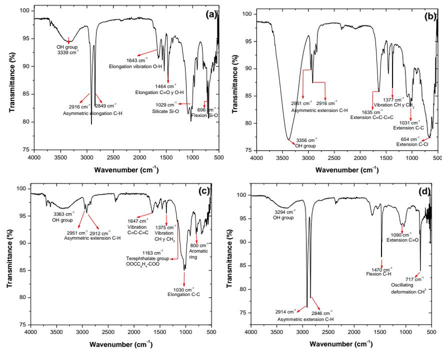
**Figure 6.** FTIR-ATR of four collected items: (a) Polyethylene + silicate (PES). (b) Chlorinated polyvinyl chloride (CPVC). (c) Polyethyleneterephthalate (PET). (d) High-density polyethylene (HDPE).
