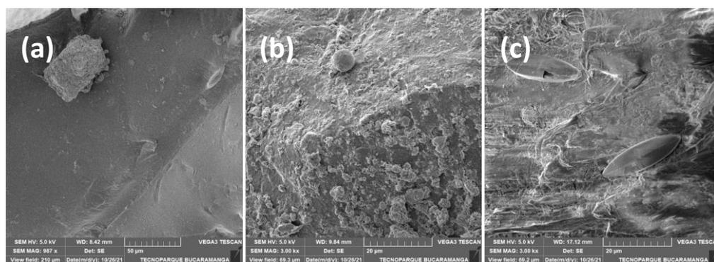
**Figure 8.** Scanning electron microscopy of microplastics (a) and mesoplastics (b,c).
