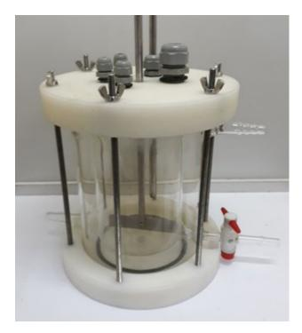
Figure 3. Complete jacketed bioreactor developed.
