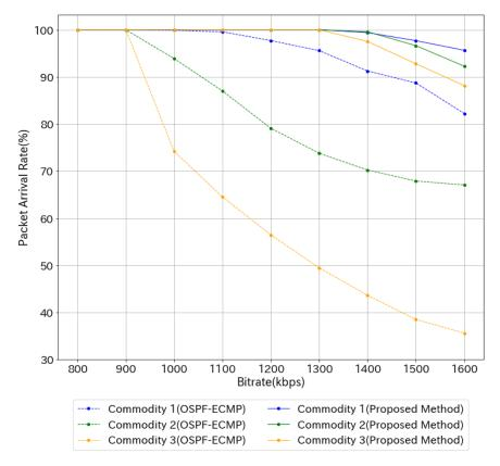
Figure 11. Packet arrival rate for 3 sources and 3 destinations.
