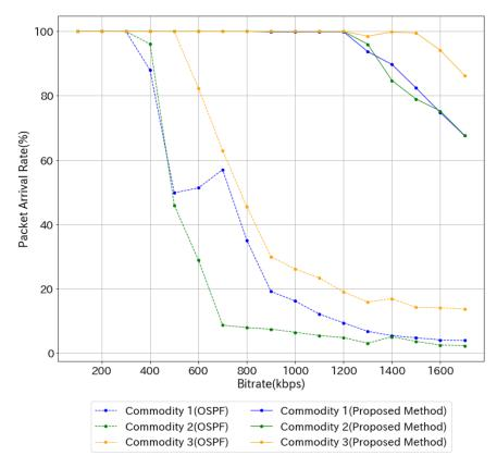
Figure 10. Packet arrival rate for 3 sources and 3 destinations.
