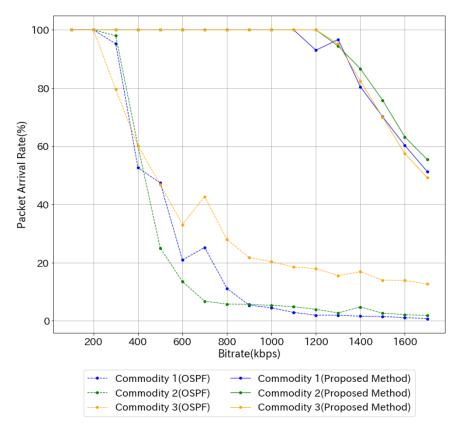
Figure 9. Packet arrival rate for 3 sources and 1 destination.
