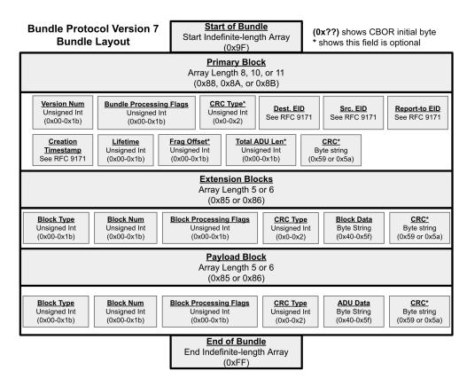
**Figure 5.** Layout of BPv7 bundles. A bundle is encoded as an indefinite–length array of blocks, and blocks are encoded as definite–length arrays of fields. The size of each field is determined by its data type and defined length in its initial byte (shown in parentheses).
