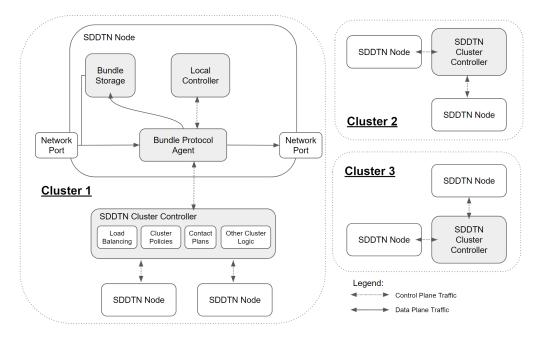
**Figure 6.** A Software-Defined Delay Tolerant Network architecture, with three clusters, each containing an SDDTN controller managing SDDTN nodes via control plane links. A SDDTN node has all the behaviors of a typical DTN node, dictated by the abstract Bundle Protocol Agent, and also has communication with a local controller.
