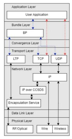
**Figure 1.** Bundle Protocol network stack. Blue dotted lines show OSI model layer 4 and up for a typical DTN network stack. Red dashed lines show the typical layer 4 and up for Earth communications (without BP). Black solid lines show the underlying network layers.
