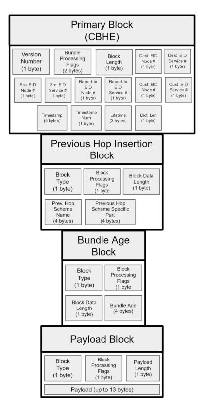
**Figure 9.** Expected format for incoming BPv6 bundles. A Previous Hop Insertion Block and Bundle Age Block are the only extension blocks expected, in this specific order. Additionally, currently only payloads up to 13 bytes are expected. There is undefined behavior for any bundles sent to the bundle translator that do not match this format.
