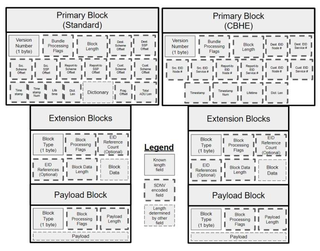
**Figure 3.** Layout of BPv6 bundles. Very few fields have a defined bit width (denoted with a solid outline). Most fields have a bit width that is only known until it is parsed using the SDNV encoded scheme (denoted with a bold dashed outline). Other fields have a width encoded by a field preceding it (denoted with a non-bold dashed outline).
