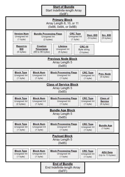
**Figure 10.** Expected format for incoming BPv7 bundles. Note that in the primary block, the creation timestamp can be between 88 to 96 bytes. A Previous Node Block, Experimental Class of Service Block, and Bundle Age Block are the only extension blocks expected, in this specific order. Additionally, currently only payloads up to 13 bytes are expected. There is undefined behavior for any bundles sent to the bundle translator that do not match this format.
