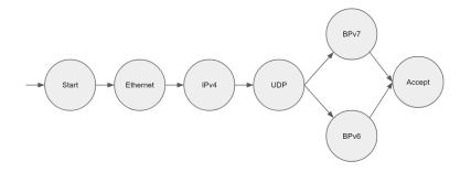
**Figure 8.** Parser state machine for Bundle Translator. The parser stage of a P4 program is coded as a series of states that are transitioned between using data from fields of the packet being parsed.
