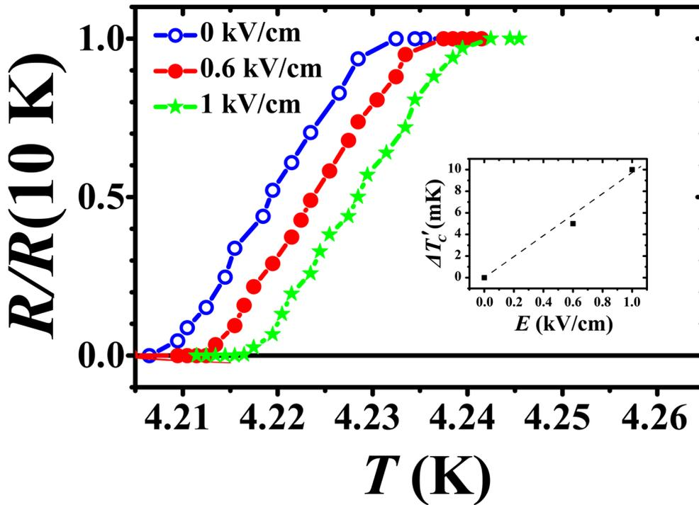
Figure 5. Superconducting transitions curves for the sample PMN-PT/Fe1(3 nm)/Cu(4 nm)/Fe2(1 nm)/Cu(1.2 nm)/Pb(60 nm)/Si<sub>3</sub>N<sub>4</sub> when applying an electric field to PMN-PT substrate.
