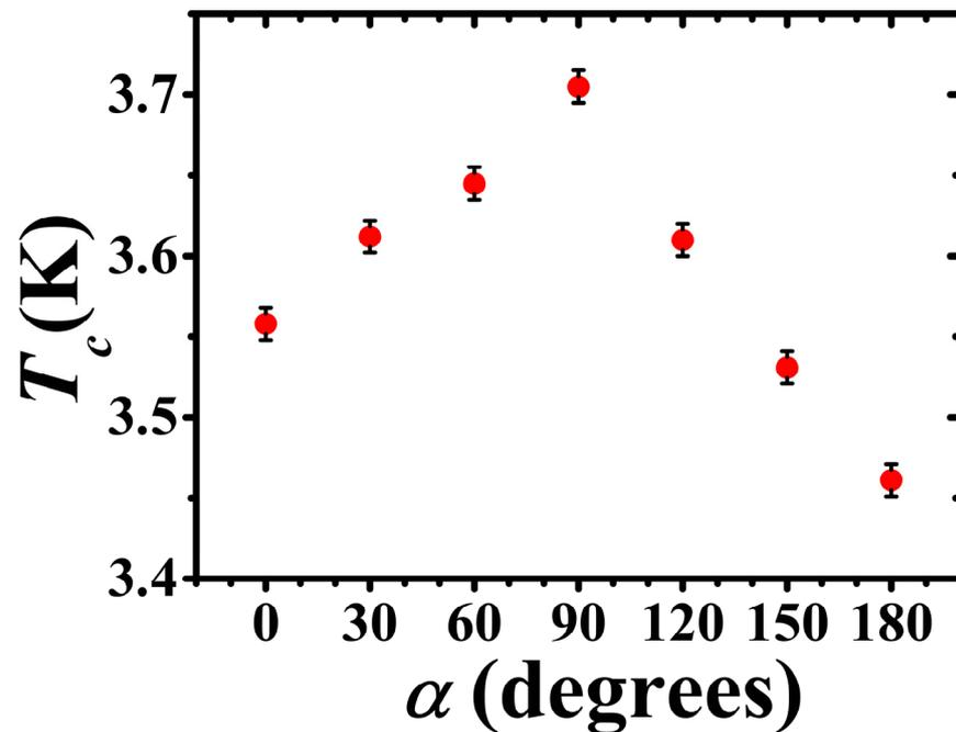
**Figure 3.** Dependence of  $T_c$  on the angle  $\alpha$  between the direction of the cooling field and the applied magnetic field  $H = 1$  kOe.
