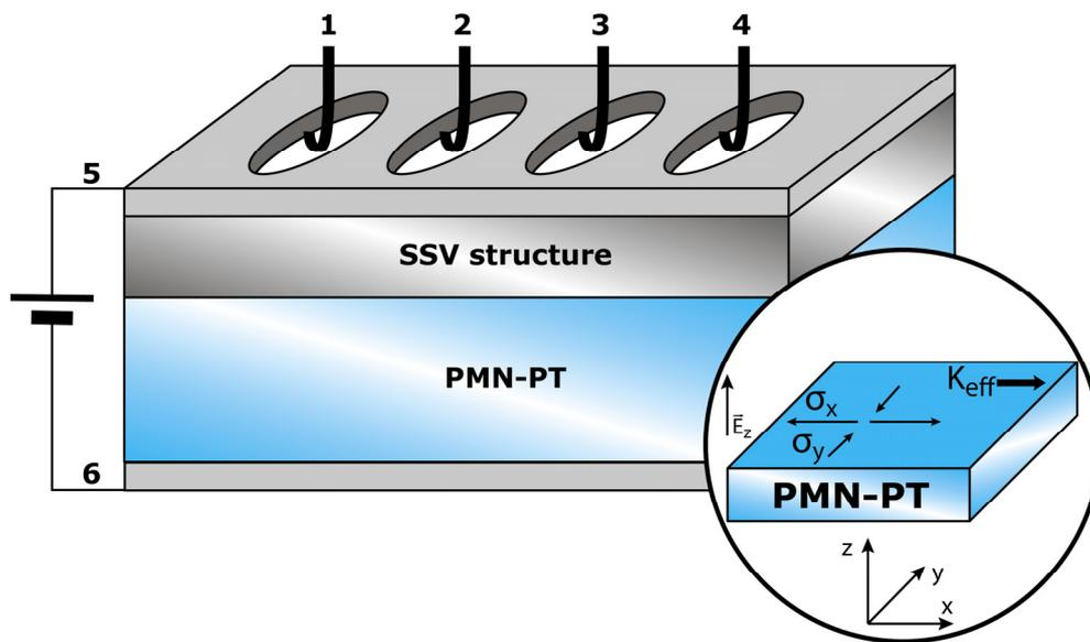
**Figure 2.** The scheme for measuring  $T_c$  by a four-probe resistivity method: 1, 4—current electrodes; 2, 3—potential electrodes; 5, 6—capacity plates for applying an electric field to a piezoelectric substrate. The inset shows the deformation of the substrate under the action of an electric field and the appearance of magnetic anisotropy with the uniaxial anisotropy constant  $K_{eff}$ .
