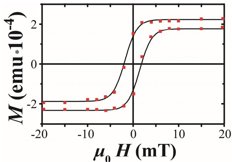
**Figure 4.** Magnetic hysteresis loop for the sample PMN-PT/Fe1(3 nm)/Cu(4 nm)/Fe2(1 nm)/Cu(1.2 nm)/Pb(60 nm)/Si<sub>3</sub>N<sub>4</sub> measured at  $T = 30$  K. The solid line is a guide for the eyes.
