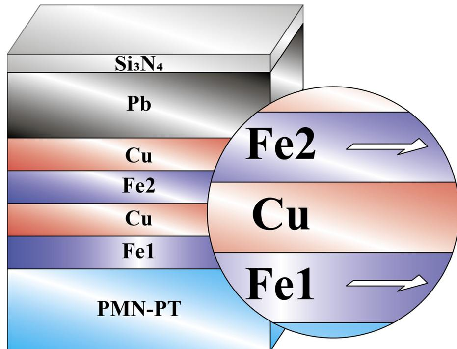
**Figure 1.** The structure of prepared SSV samples.
