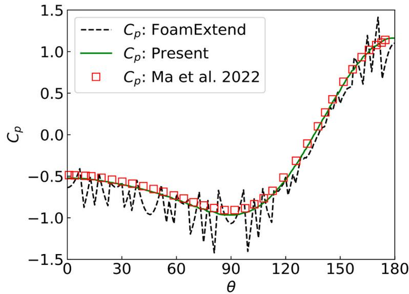
**Figure 5.** Comparison of pressure coefficient on the cylinder wall obtained using the EIB-LBFS method and the IBM in FOAM-Extend with the reference data from Ma et al. [49] for flow past a cylinder at  $Re = 40$ .
