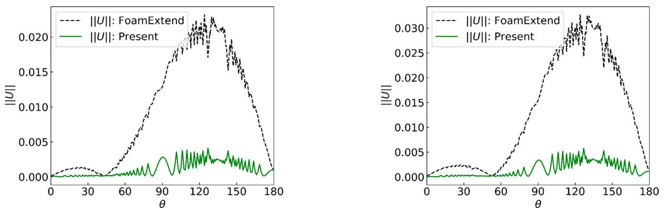
**Figure 4.** Comparison of the velocity on the cylinder surface obtained using the EIB-LBFS method and the IBM in FOAM-Extend for flow past a cylinder at  $Re = 20$  (left) and  $Re = 40$  (right).
