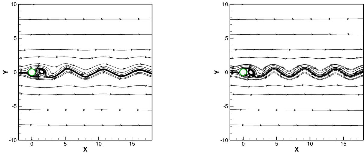
**Figure 6.** Streamlines around the cylinder obtained using the EIB-LBFS method for flow past a cylinder at  $Re = 100$  (left) and  $Re = 200$  (right).
