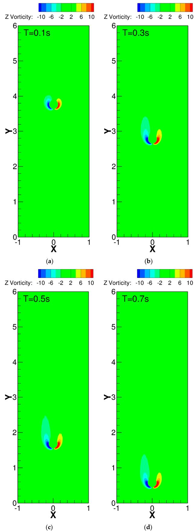
**Figure 15.** Vorticity contours at (a)  $t = 0.1$  s, (b)  $t = 0.3$  s, (c)  $t = 0.5$  s, and (d)  $t = 0.7$  s obtained using the EIB-LBFS method for the falling circular cylinder in a rectangular box.
