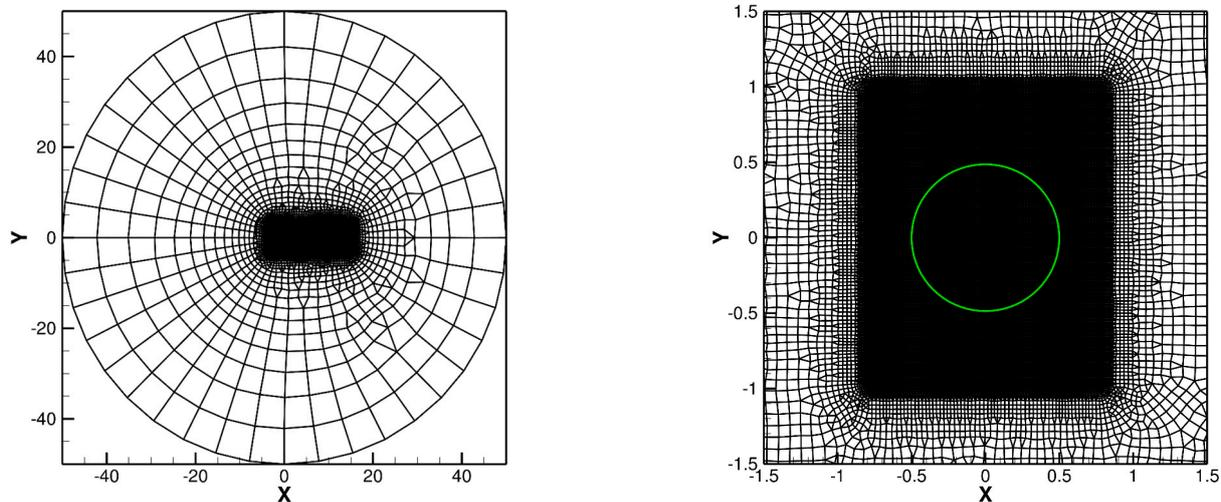
**Figure 2.** Entire unstructured mesh (left) and close-up view of the uniform mesh around the cylinder (right) for viscous flow past a circular cylinder. The cylinder boundary is represented by the green circle.
