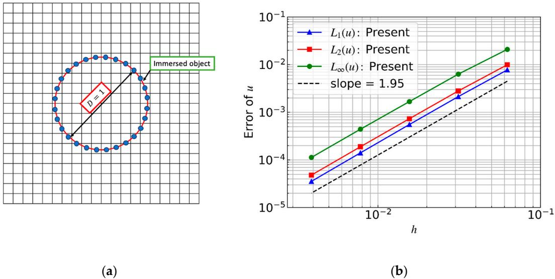
Figure 1. Spatial accuracy test of the EIB-LBFS for the Taylor–Green vortex: (a) schematics of the simulation and (b) convergence history of errors with mesh refinement.
