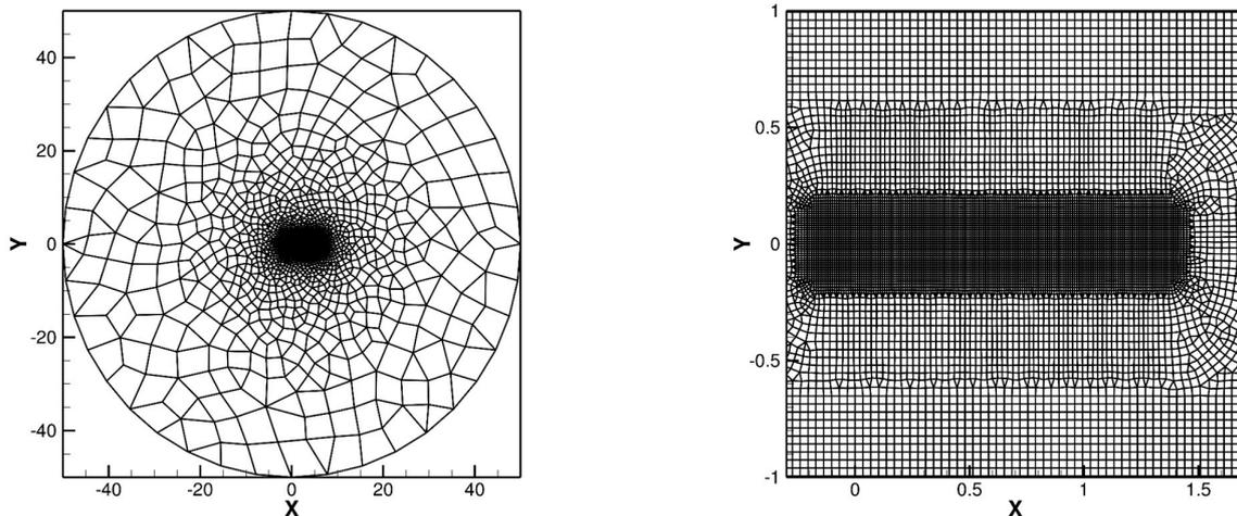
**Figure 8.** Entire unstructured mesh (left) and close-up view of the uniform mesh around the airfoil (right) for flow past a stationary NACA-0012 airfoil at  $Re = 500$ .
