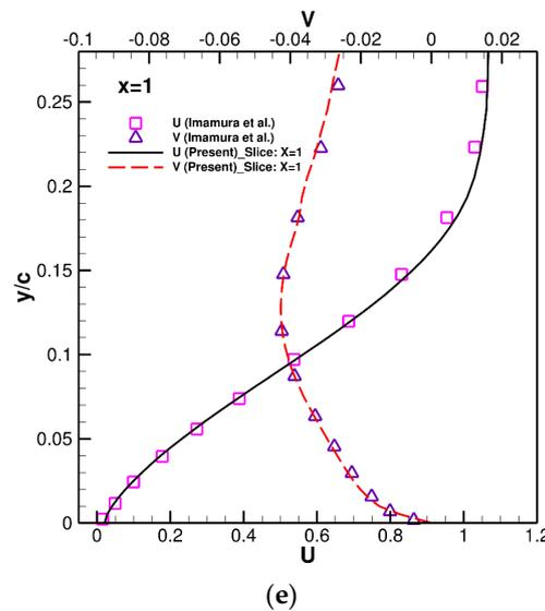
**Figure 11.** Comparison of  $u$ -velocity and  $v$ -velocity profiles at (a)  $x = 0.00$ , (b)  $x = 0.25$ , (c)  $x = 0.50$ , (d)  $x = 0.75$ , and (e)  $x = 1.00$  obtained using the EIB-LBFS method with reference data reported by Imamura et al. [59] for flow past a stationary NACA-0012 airfoil at  $Re = 500$ .
