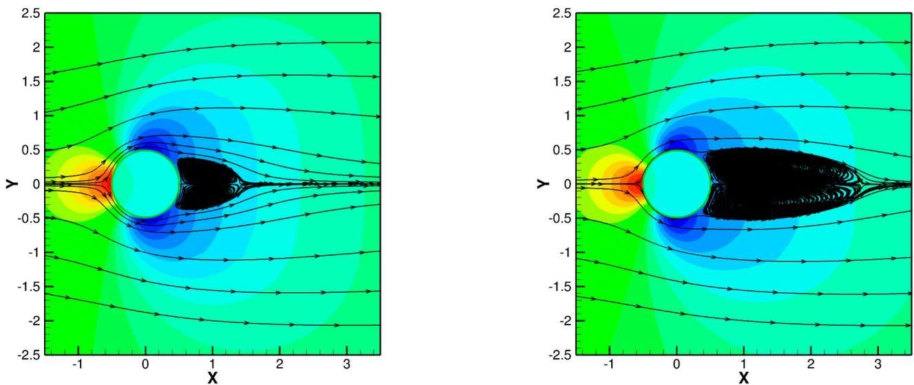
**Figure 3.** Pressure contours and streamlines around the cylinder obtained using the EIB-LBFS method for flow past a cylinder at  $Re = 20$  (left) and  $Re = 40$  (right).
