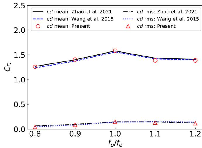
**Figure 12.** Comparison of the computed mean drag coefficient and root-mean-square value of drag coefficient with the reference data from Wang et al. [37] and Zhao et al. [30] for flow past an oscillating circular cylinder.
