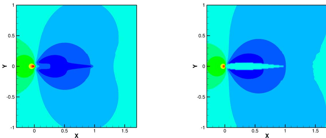
**Figure 9.** Comparison of pressure contours around the airfoil obtained using the EIB-LBFS method (left) and the IBM in FOAM-Extend (right) for flow past a stationary NACA-0012 airfoil at  $Re = 500$ .
