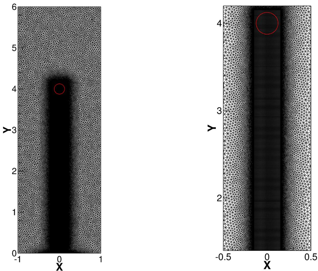
**Figure 14.** Entire mesh (left) and close-up view of mesh in the region along the sedimentation trajectory (right) for sedimentation of a circular particle in a rectangular box. The solid boundary of the circular particle is represented by the red circle.
