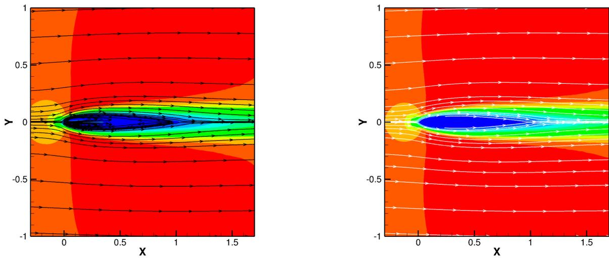
Figure 10. Comparison of  $u$ -velocity contours and streamlines around the airfoil obtained using the EIB-LBFS method (left) and the IBM in FOAM-Extend (right) for flow past a stationary NACA-0012 airfoil at  $Re = 500$ .
