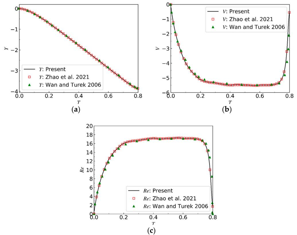
**Figure 16.** Comparison of the time evolution of (a) vertical coordinate, (b) vertical velocity, and (c) local Reynolds number obtained using the EIB-LBFS method with reference data from Zhao et al. [30] and Wan and Turek [62] for sedimentation of a circular particle in a rectangular box.
