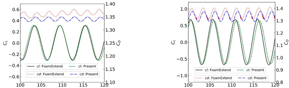
**Figure 7.** Comparison of evolution of the lift and drag coefficients obtained using the EIB-LBFS method and the IBM in FOAM-Extend for flow past a cylinder at  $Re = 100$  (left) and  $Re = 200$  (right).
