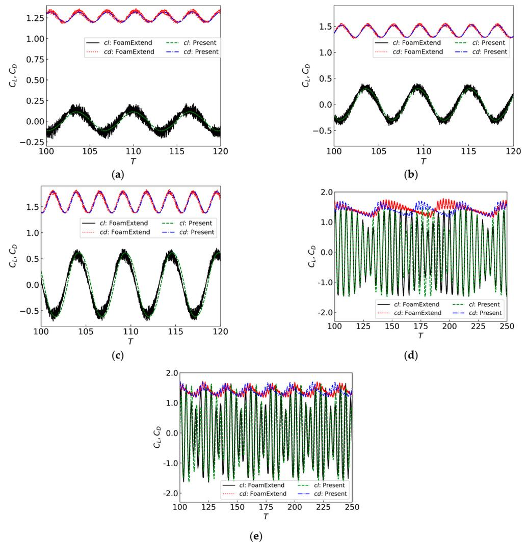
**Figure 13.** Comparison of lift and drag coefficients for flow past an oscillating circular cylinder: (a)  $f_e/f_o = 0.8$ , (b)  $f_e/f_o = 0.9$ , (c)  $f_e/f_o = 1.0$ , (d)  $f_e/f_o = 1.1$ , and (e)  $f_e/f_o = 1.2$ .
