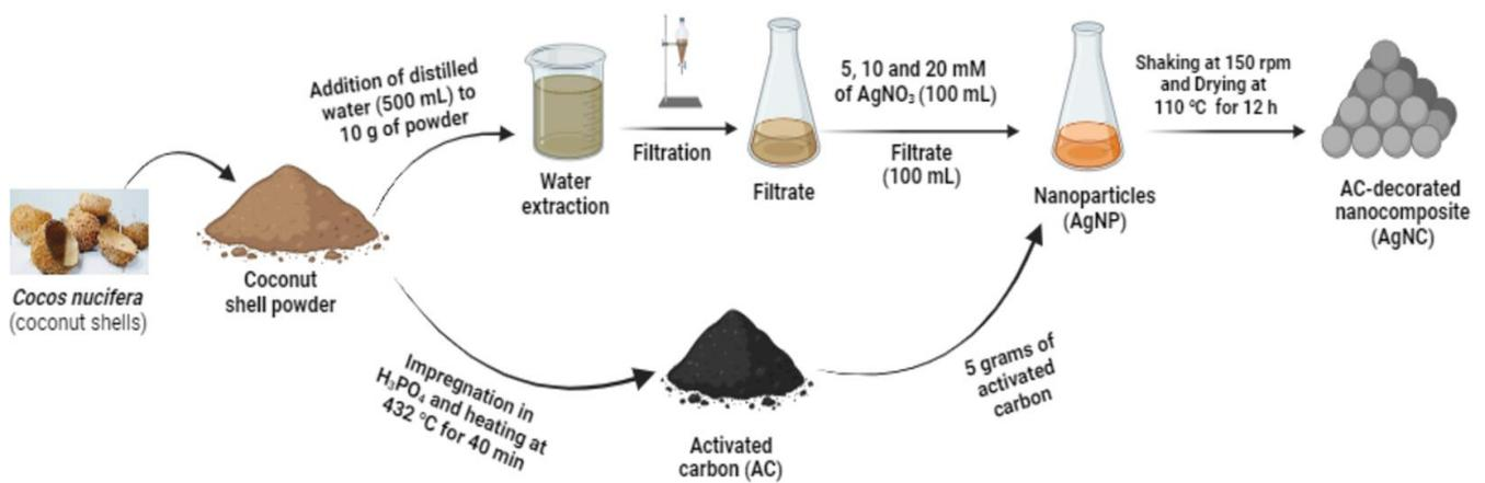
**Figure 1.** Graphical representation of the preparation of extract, silver nanoparticles, and nanocomposites from *Cocos nucifera* shells.
