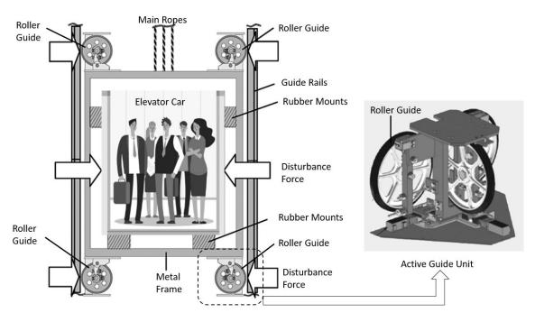
Figure 5. Computerized roller guides system. (Source: author).
