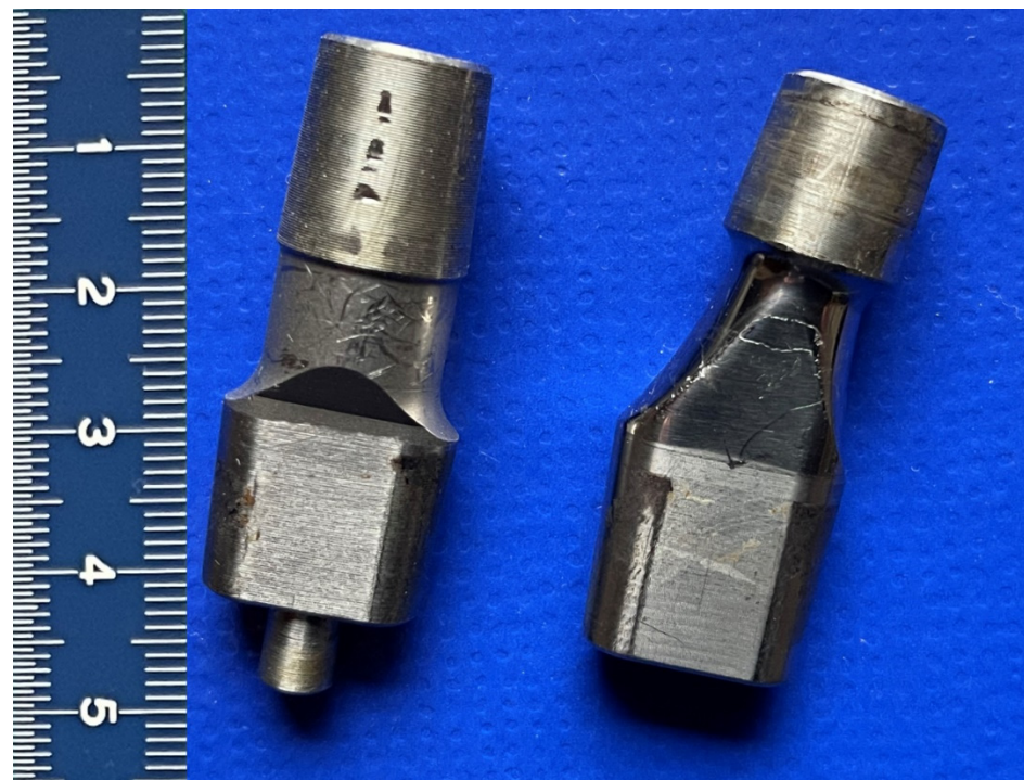
Figure 1. The exchangeable neck of the GSP (Cremascoli S.p.A.) (left) and Profemur Z (Wright Medical Technology Inc.) (right) dual-modular systems. Both necks are short, the GSP-neck is straight, and the Profemur Z-neck is in an 8^\circ varus orientation. Note the same dimensions of the rectangular-shaped cross section with rounded fillets of the distal Morse taper [6].
