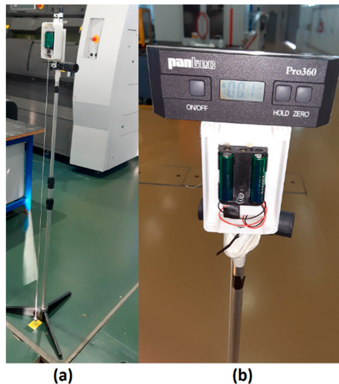
Figure 7. (a) Positioning the tag over a reference point with the center plumb. (b) Tag leveling with digital protractor.
