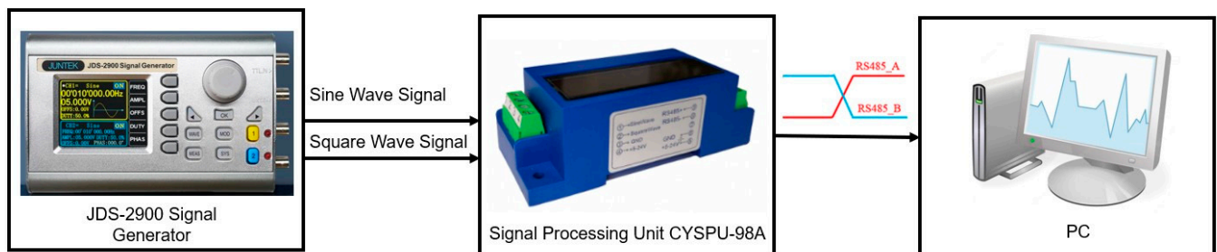
Figure 8. Block diagram of the signal generator-based frequency test system.
