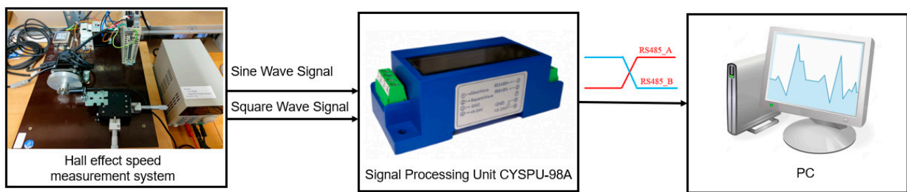
Figure 11. Block diagram of a Hall effect gear tooth sensor-based frequency test system.
