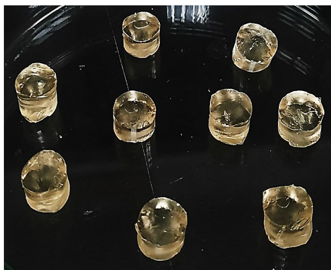
Figure 2. The physical appearance of PEG-co-p(AAc/AMPS) hydrogel discs.
