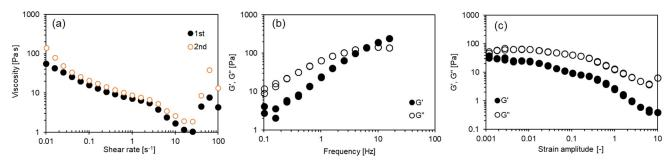
**Figure 3.** Viscosity, storage modulus (G'), and loss modulus (G'') of climbing colloidal suspension of 70 wt. % silica particles of 1.0 µm diameter and water: (**a**) viscosity against shear rate, (**b**) G' and G'' against frequency at a strain amplitude of 0.01, and (**c**) G' and G'' against strain amplitude at a frequency of 1 Hz.
