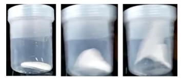
**Figure 1.** Pictures of the climbing colloidal suspension of 70 wt. % silica particles of 1.0  $\mu$ m diameter with water under horizontal vibration. The corresponding movie is given in Supplementary Materials. The left picture shows the suspension at rest, and the middle (~8 s in the movie) and right (~12 s in the movie) ones are under vibration.
