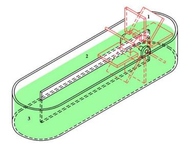
Figure 1. Scheme of open photobioreactor: (1) paddle wheel; (2) pond area; (3) baffle.
