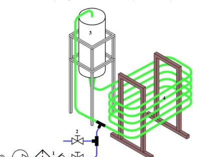
(Figure 2); manifold; helical; and fence arrangement with manifold photobioreactors [77], where the tubes may be positioned horizontally or vertically for maximal solar capture [7].
