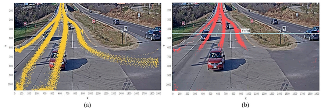
Figure 1. Stopbar identification process from vehicle trajectories at a sample intersection approach: (a) trajectory points, (b) stopped locations (red points) and the stopbar line.
