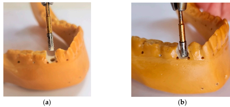
Figure 4. (a,b) BKS with the bone graft inside its inner volume implanted in the surgical alveolus created.
