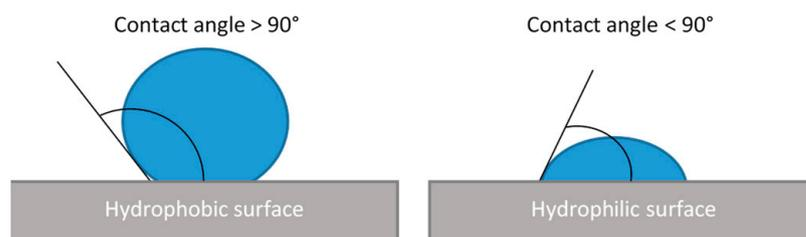
**Figure 3.** Schematic representation of hydrophobic and hydrophilic surfaces.
