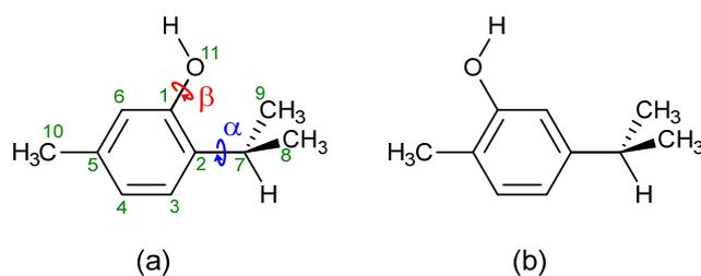
**Scheme 1.** Molecular structures of thymol (a) and carvacrol (b), including numbering of the heavy atoms and identification of the two conformationally relevant dihedral angles for the thymol structure. The H atoms connected to the aromatic ring are implicit.
