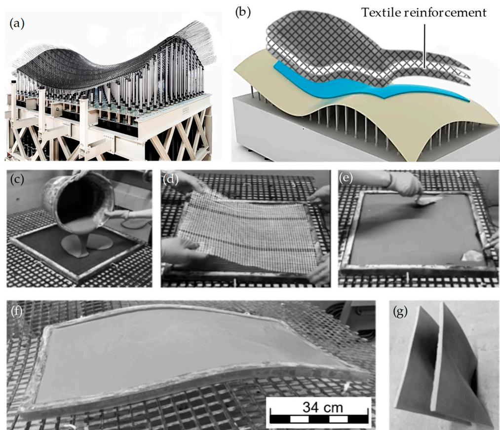
**Figure 12.** Precasting of TRC with adaptive mold at ITA: (a) industry-scale adaptive mold form ADAPA AS; (b) schematic; (c) filling silicon mold with first layer of concrete in flat position; (d) placement of textile reinforcement; (e) pouring second layer of concrete; (f) deforming on the adaptive mold; (g) precast TRC panels.
