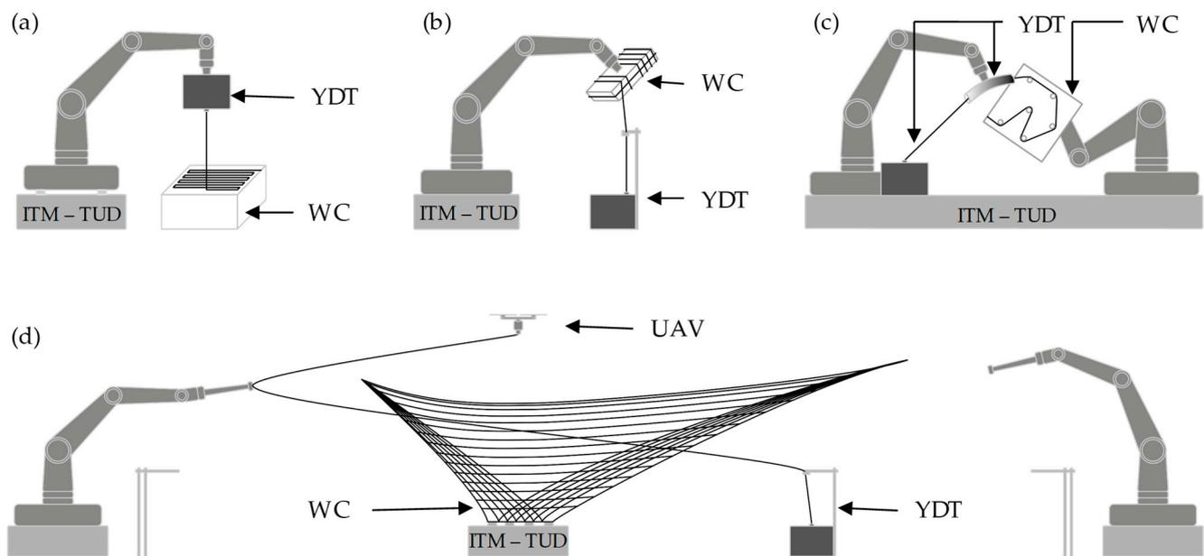
**Figure 10.** Robot-assisted yarn deposition principles: (a)—process principle A; (b)—process principle B; (c)—process principle C; (d)—process principle D; WC = workpiece carrier, YDT = yarn deposition tool, UAV = unmanned aerial vehicle [80,81,83,87,89,92,93].
