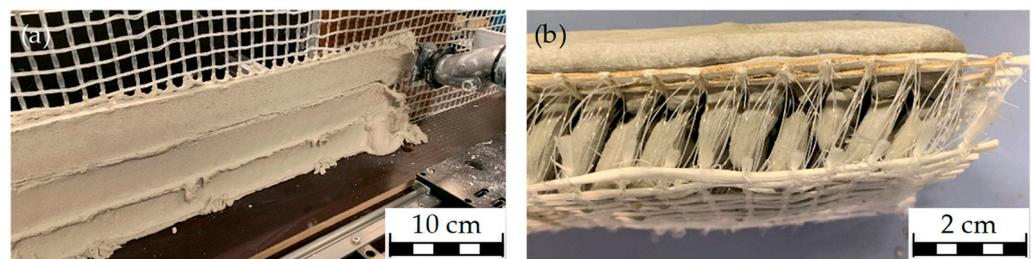
**Figure 13.** Two approaches for the textile reinforcement of 3D concrete printing: (a) printing through a two-dimensional, grid like textile; (b) specimen made by printing onto a three-dimensional spacer fabric.
