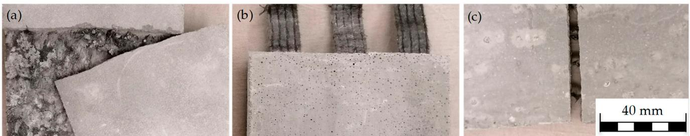
**Figure 15.** Variations in using rCF as textile reinforcement in concrete: (a) rCF nonwoven reinforcement occurs as a separating layer; (b) nonwoven reinforcement inserted in stripes; and (c) rCF hybrid yarn reinforcement.
