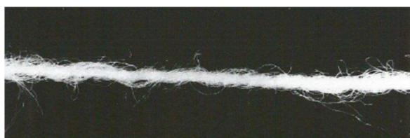
**Figure 4.** The world's first yarn spun in a rotor.
