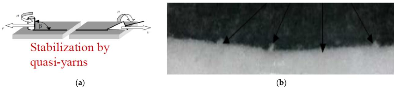
Figure 14. Surface quasi yarns on surface of ROTIS structures (a) principle of forming and (b) appearance.
