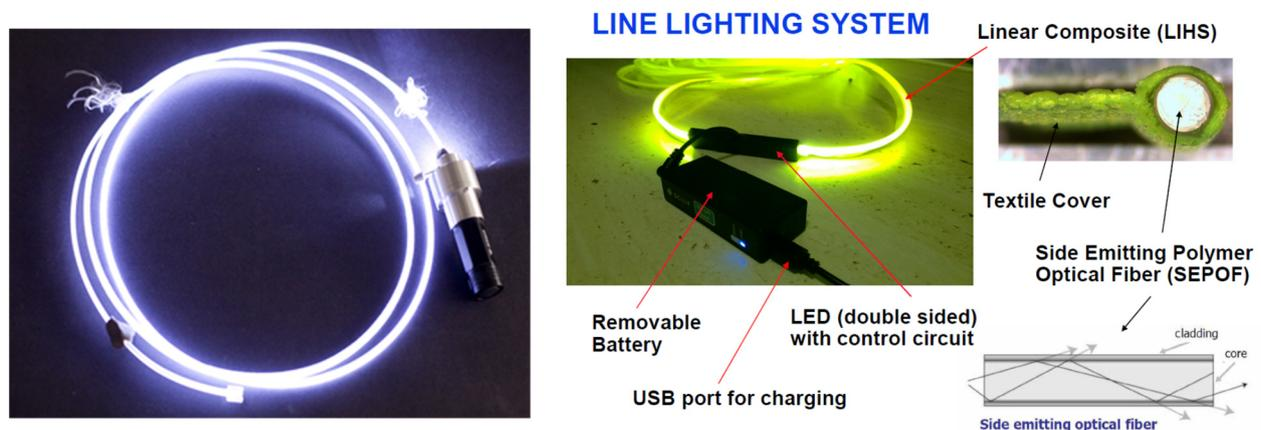
**Figure 1.** Structure of SEPOF and line lighting system.
