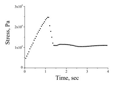
Figure 3. Typical stress versus time curve for PDADMAC100. Traverse rate 5 mm/min.
