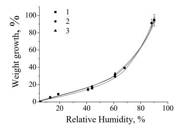
**Figure 2.** Dependence of the coating formed from PDADMAC 100 (1), PDADMAC 200 (2) and PDADMAC 400 (3) weight on the relative humidity.
