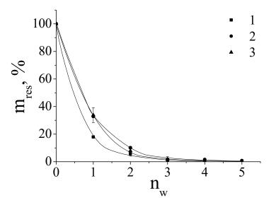
**Figure 1.** Dependence of the percentage of residual mass of coatings ( $m_{res}$ ) formed from PDADMAC 100 (1), PDADMAC 200 (2) and PDADMAC 400 (3) on the number of wash-off cycles ( $n_w$ ).
